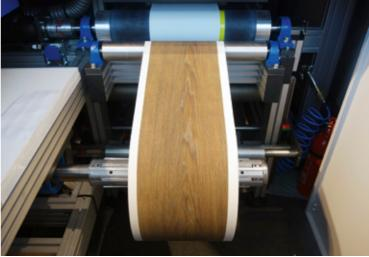
Fagus-Grecon's new generation of "Superscan" systems can distinguish between real defects and "pseudo defects".
